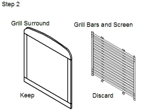
Remove Grill Bars and Screen from grill frame and discard. Keep the outer surround. You will be mounting the punched grill to it
